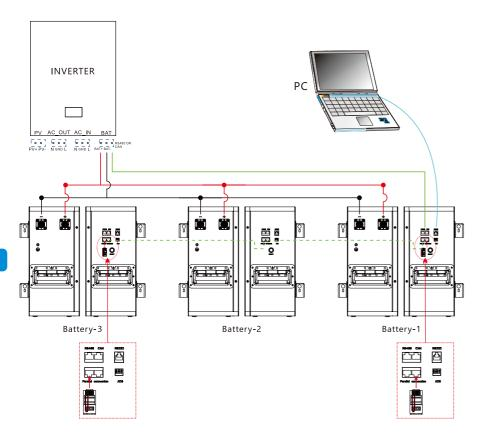
NOTE: The powerlines between each battery are the same length.
